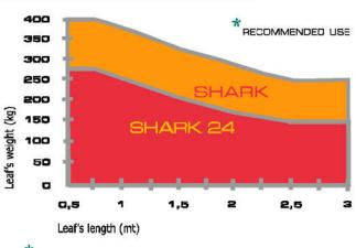
Exposure to high winds, the type and the shape of the gaze may all significantly reduce the usage limits.
